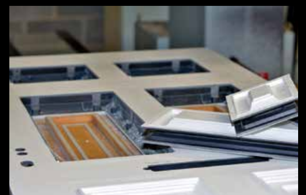
Door after routing operation
