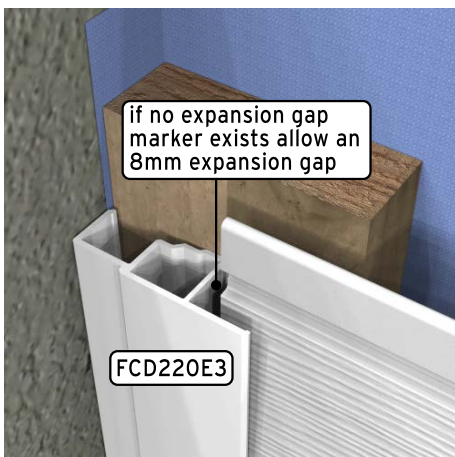
Typical Edge Detail - Multifunction Trim
